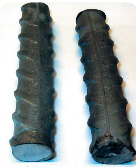
Fig. 7 Rebars of S32101 after exceeding the breakdown potentials in pore solution containing a) 1 g/L chlorides and b) 10 g/L chlorides.
