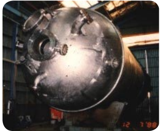
Fig. 3 A kraft batch digester made of 2205.
