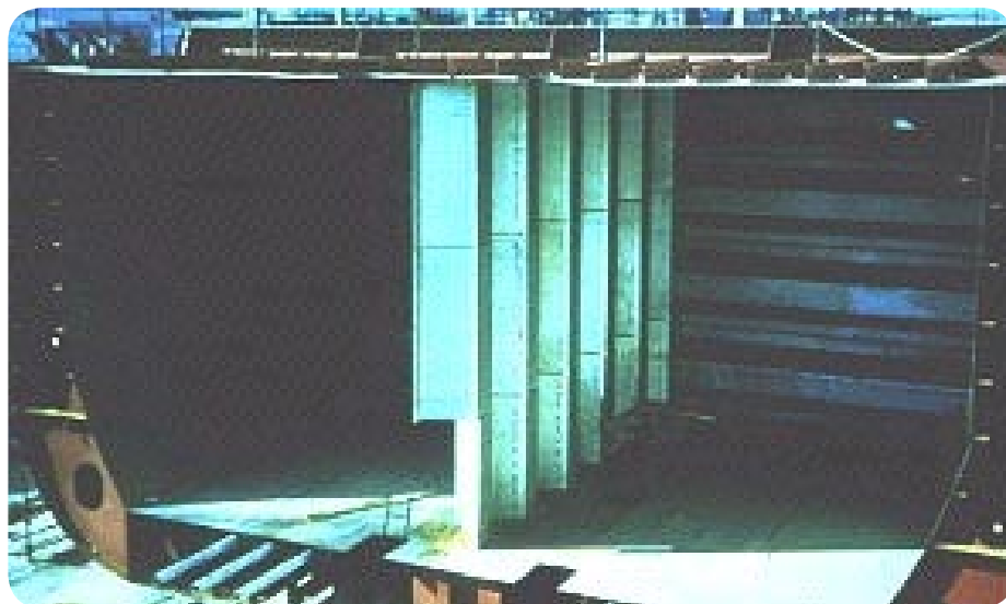
Fig. 6 Chemical tanker with 2205 tanks under construction.
